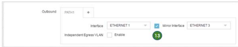
Figure 13: Configuration – Mirror Interface configuration
